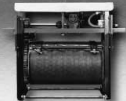
Model 2MSTXOMC 15"x26" gear driven, round, mild steel, barrel. Cylinder is constructed of 12 ga. mild steel with 1/8" perforations. The overhead 1/4 HP fixed speed motor delivers a cylinder speed of 2RPM. The barrel has a Self Standing hangerarm arrangement. A full length polypropylene hood protects components from the drippings of passing barrels.
