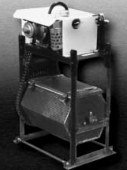
Model 2MSTBPMC 12"x18" chain driven barrel is constructed of 12 ga. steel. The hex cylinder has 1/4" perforations. The variable speed overhead air motor delivers a cylinder speed of 2-5 RPM. The barrel has a Self Standing hangerarm arrangement.
