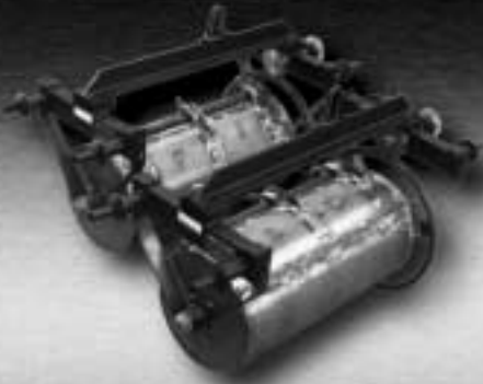
Two Model 2MMUSD 14"x30" gear driven round barrels. Cylinders are constructed of 12 ga. Monel with 1/8" perforations. A 96 tooth cylinder ring provides a 4.6:1 ratio. Upper superstructures are protection coated, mild steel. The barrels are tank supported with a Strap hangerarm arrangement.
