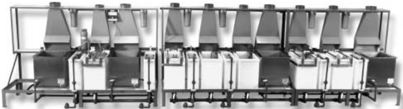
Modularized, 16 Station Cleaning Line complete with spray rinses, electro-cleaners, heaters and controls, pumps, filters, ventilation hoods, water feeds, and drains. Natural polypropylene flanged tanks feature heat bent corners, fusion welded seams, and extrusion welded bottoms. Stainless steel tanks are incorporated into the system.
