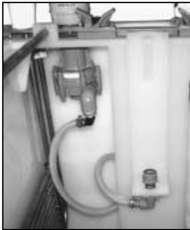
A switch on the tank saddle activates the submersible pump when the barrel is seated on the Z-bracket coupling
