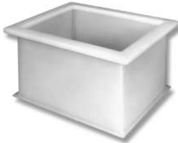
Rectangular Poly Tank, standard one (1) piece wall construction, bent corners, extrusion welded bottom, 1" top flange.
