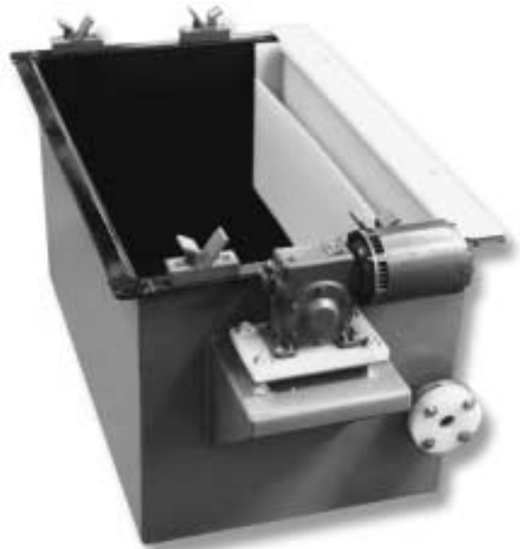
Steel/Koroseal Lined Rinse Tank, with field adapted polypropylene overflow dam.
